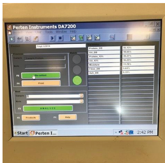
Figure 1. NIR instrument used to measure protein and oil.
