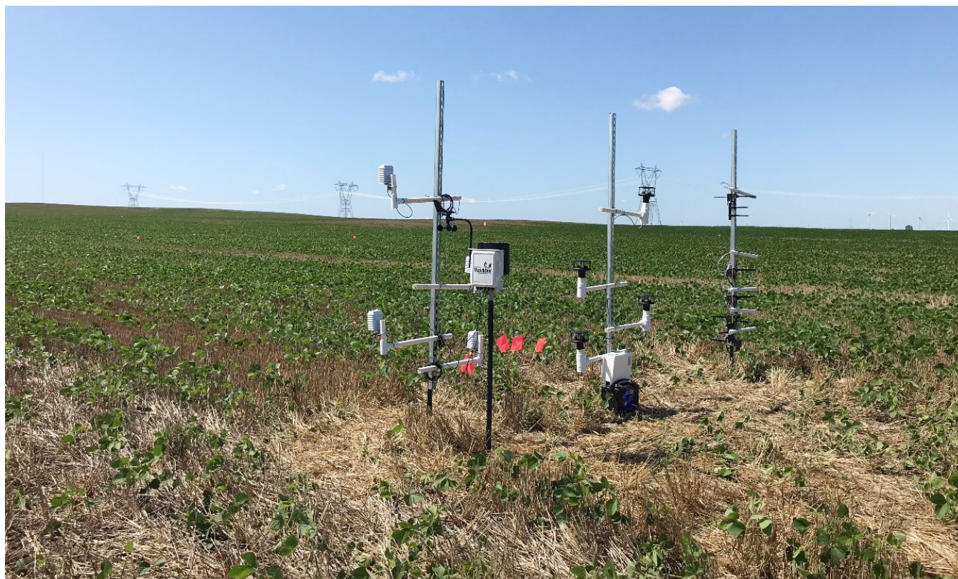
Figure 1. Weather instruments and air samplers involved with large-scale research for off-target movement of herbicides.
