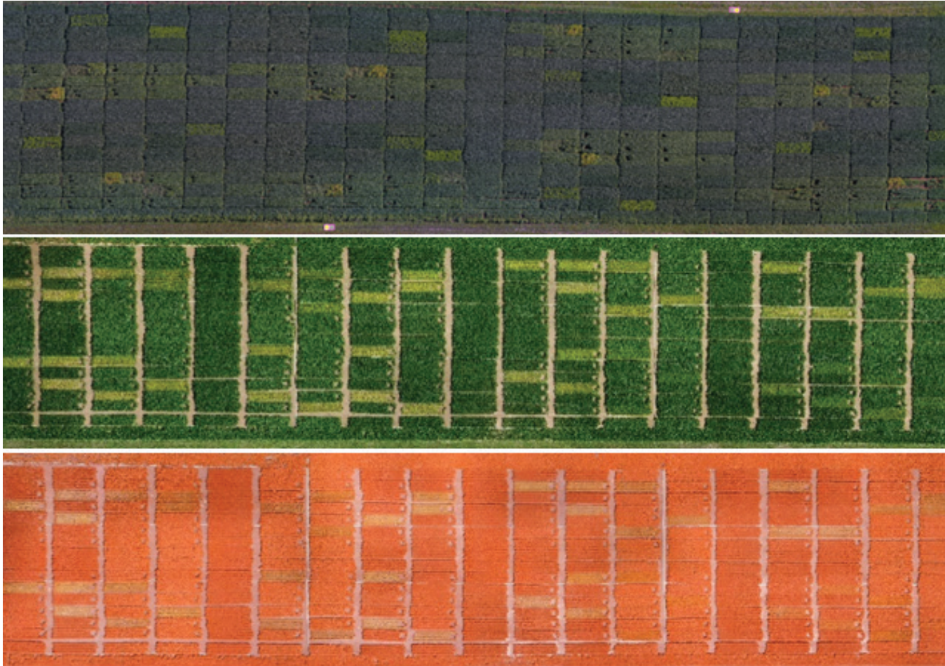
Figure 1. Aerial images of experimental plots collected in Kentucky (top) and in Arkansas (middle and bottom) during the soybean growing season, which were sampled for various laboratory analyses related to nitrogen status. The bottom panel is the normalized difference vegetation index (NDVI) using near infrared (NIR); the NDVI has arbitrarily been assigned an orange color in this image.
