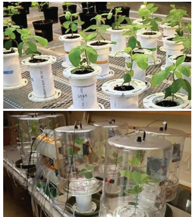
Figure 1. Measuring whole plant transpiration rate under high evaporative demand (dry air: > 2.5 kPa) in 2019.
